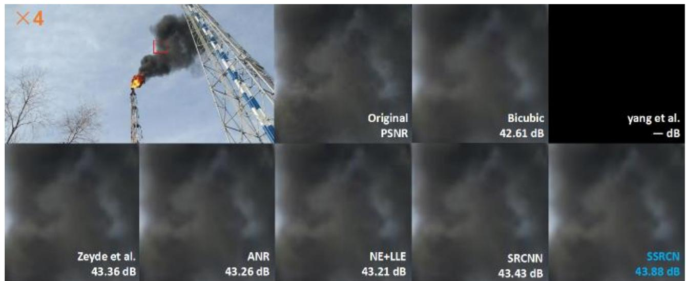
Figure 4: Flare stack scene image with an upscaling factor 4. Black smoke block diagrams in the red frame area of the original image, and marked the PSNR of the corresponding block. (The Yang et al. source program cannot be used for 4x upsampling.)
