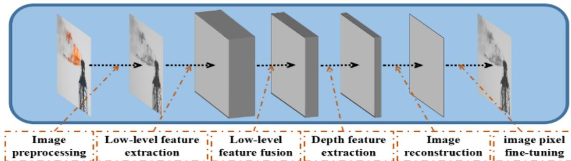
Figure 1: The algorithm flow of our proposed smoke image super-resolution method.
